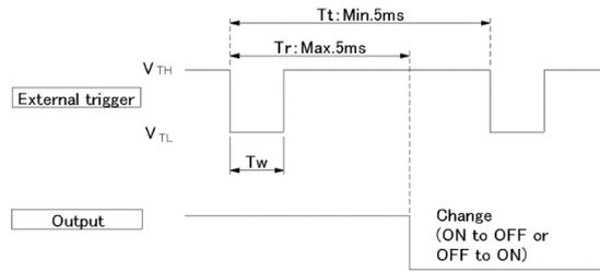
Note: The sensor recognizes at the  $V_{TH} \rightarrow V_{TH}$  edge of an external trigger that the external trigger has been input.
