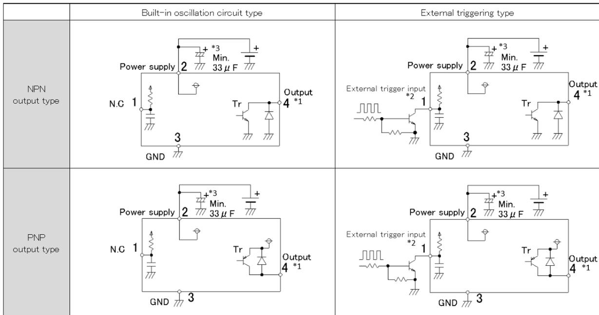
Note: \*1. The output transistor has an open collector structure.
